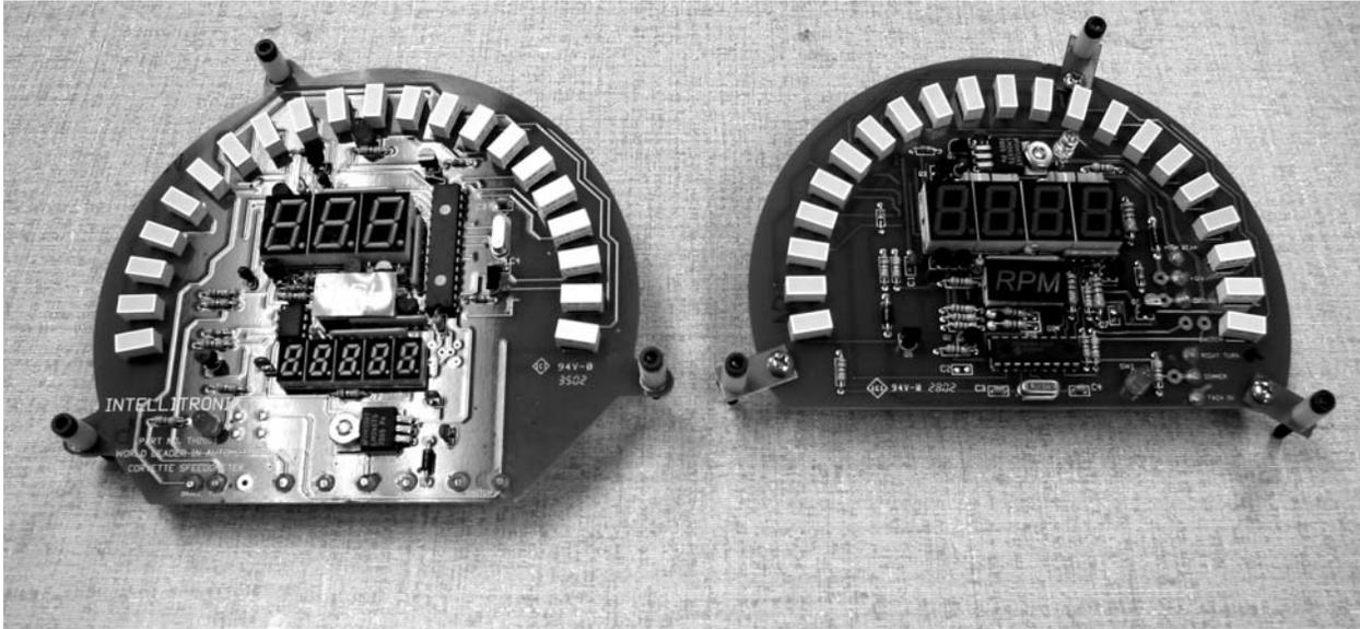
Pictured above are the speedo and tach boards with the included mounting hardware assembled on both boards. The 6/32 nuts are mounted on the backside of both boards on each of the screws. The three rectangular extender tabs used on the tach board may not be needed for all applications.
