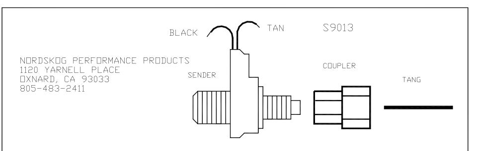
IT IS ADVISABLE TO KEEP ALL WIRES AWAY FROM IGNITION WIREIGNITION WIRES WILL CAUSE ERRATIC READINGS.
